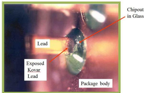
Reject.. A significant chipout in the glass to metal seal which exposes the base Kovar metal on the lead.
